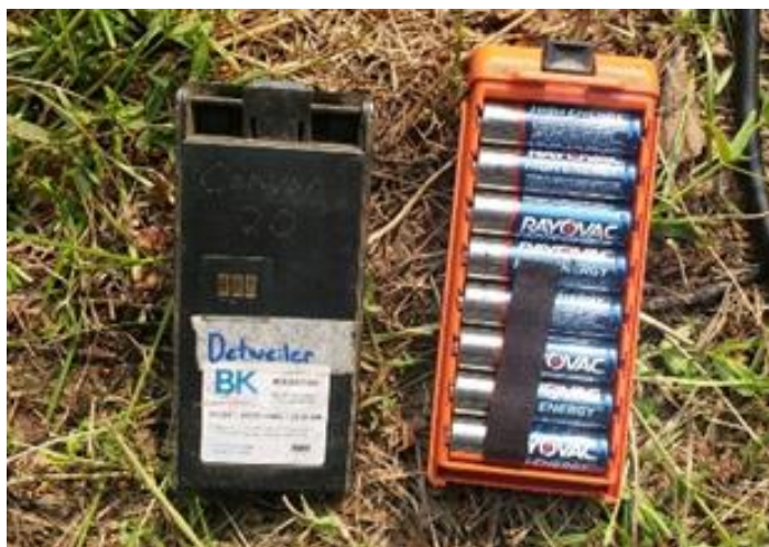
Closeup of Rechargeable Clamshell vs Alkaline AA Clamshell on the Nez Perce-Clearwater NF. USDA Forest Service photo by Mark Wahlberg, USDA FS.
