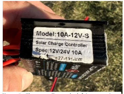
Figure 5- The controller on the left is a generic 12- or 24-Volt automatic unit capable of 10 Amps, with an SLA battery. It's waterproof and simple and will handle a single solar panel. It will regulate a 12 Volt SLA to about 13.5-13.6 Volts. This was an eBay purchase, about $12 delivered.
