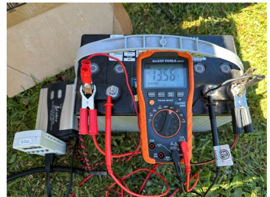
Figure 14 A battery not fully charged.
