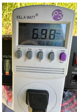
Figure 12 This is reading the real time power delivered to the coffee pot: 785 Watts (112.6 Volts times 6.98 Amps).
