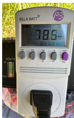
Figure 11 Plug either an outlet strip or heavy-duty extension cord into the Kill-A-Watt to distribute power (6.98 Amps AC to power the coffee pot).
