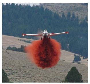
lead aircraft dropped the full retardant load and began a shallow climbing left turn. The trailing aircraft was observed to remain below the lead aircraft, flying through the lead's retardant. With retardant covering the windscreen, the pilot released the full retardant load and initiated a rapid, climbing left turn into the lead aircraft.
