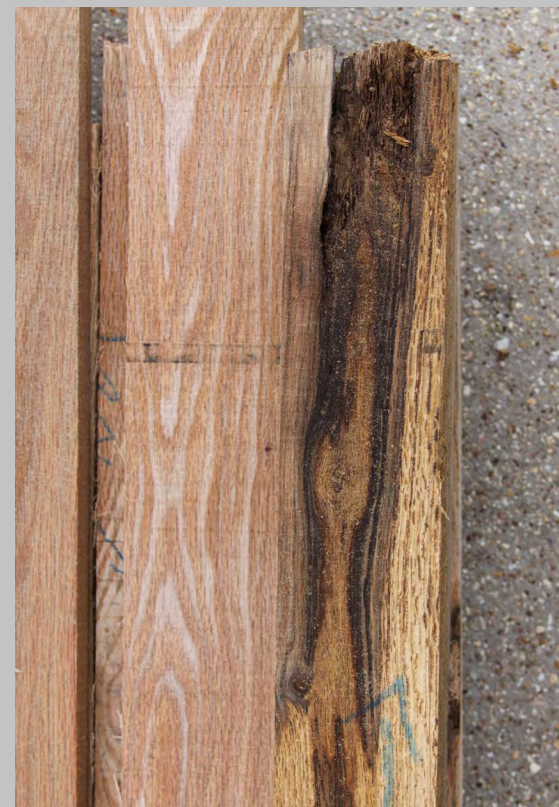
Figure 6 —Decay and stain associated with a fire-scarred red oak in Missouri, defects in the wood that developed within 15 years of the fire injury. Photo: Dan Dey, USDA Forest Service, Northern Research Station.
