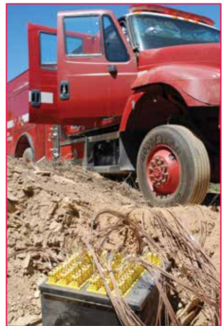
Data collection device and sensor connecting wires are prepared for installation in and on fire engines. Photo by Ryan Myers, 2013.
