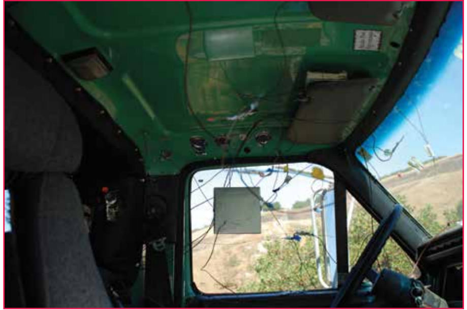
Sensors are mounted inside the cab of a fire engine to gather data during the burn. Photo by Ryan Myers, 2013.
