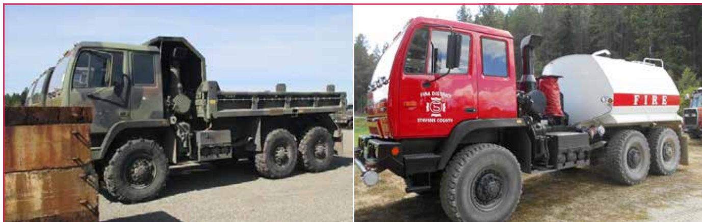
An M-1090 military dumptruck (left) acquired by Stevens County Fire District #5 through the Washington State Department of Natural Resources Firefighter Property Program and converted into a water tender for wildland firefighting (right). Photo: Washington State Department of Natural Resources.
