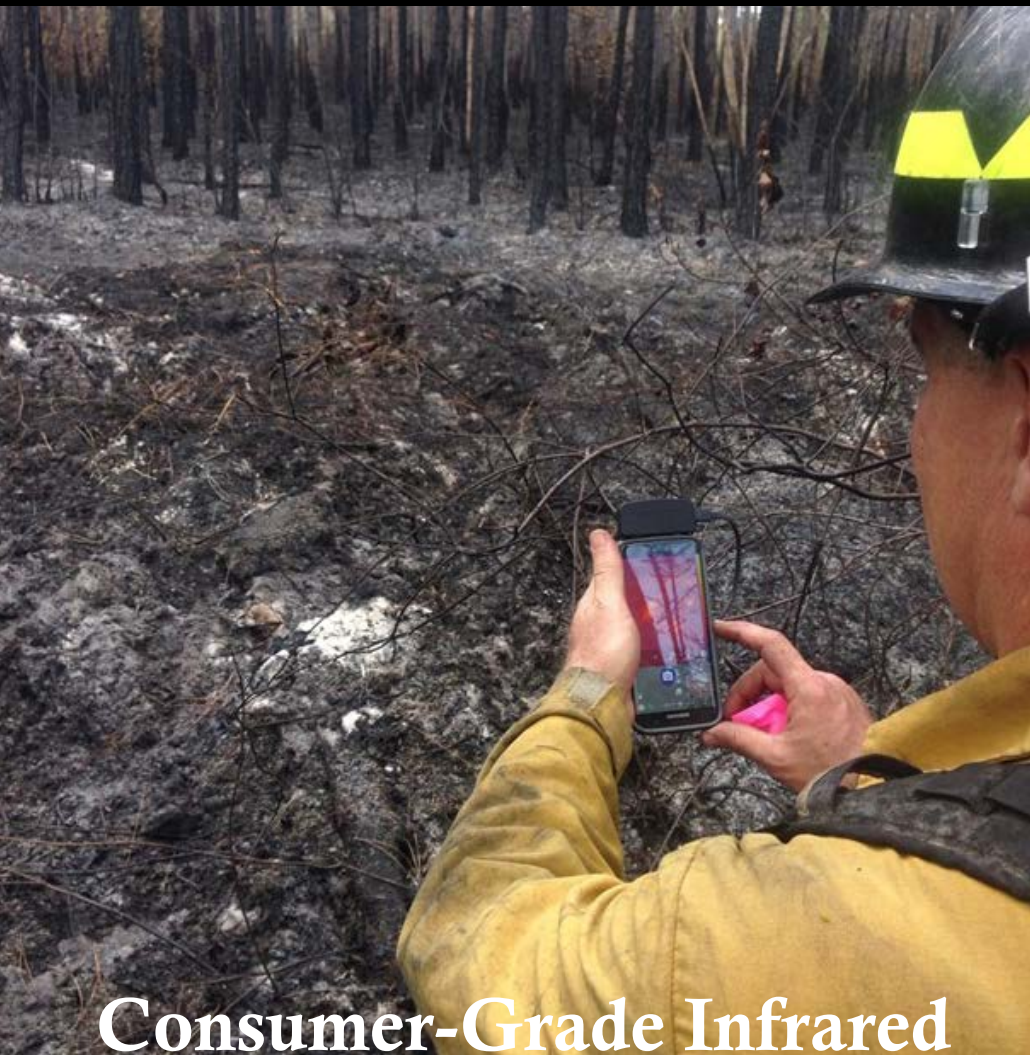
Figure 1 —The FLIR-One thermal imaging system being tested on an obvious hotspot. Photo: Joe O'Brien, USDA Forest Service.
