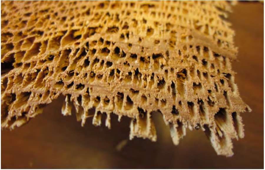
Figure A1.27—Honeycombed decay caused by Onnia tomentosa .
