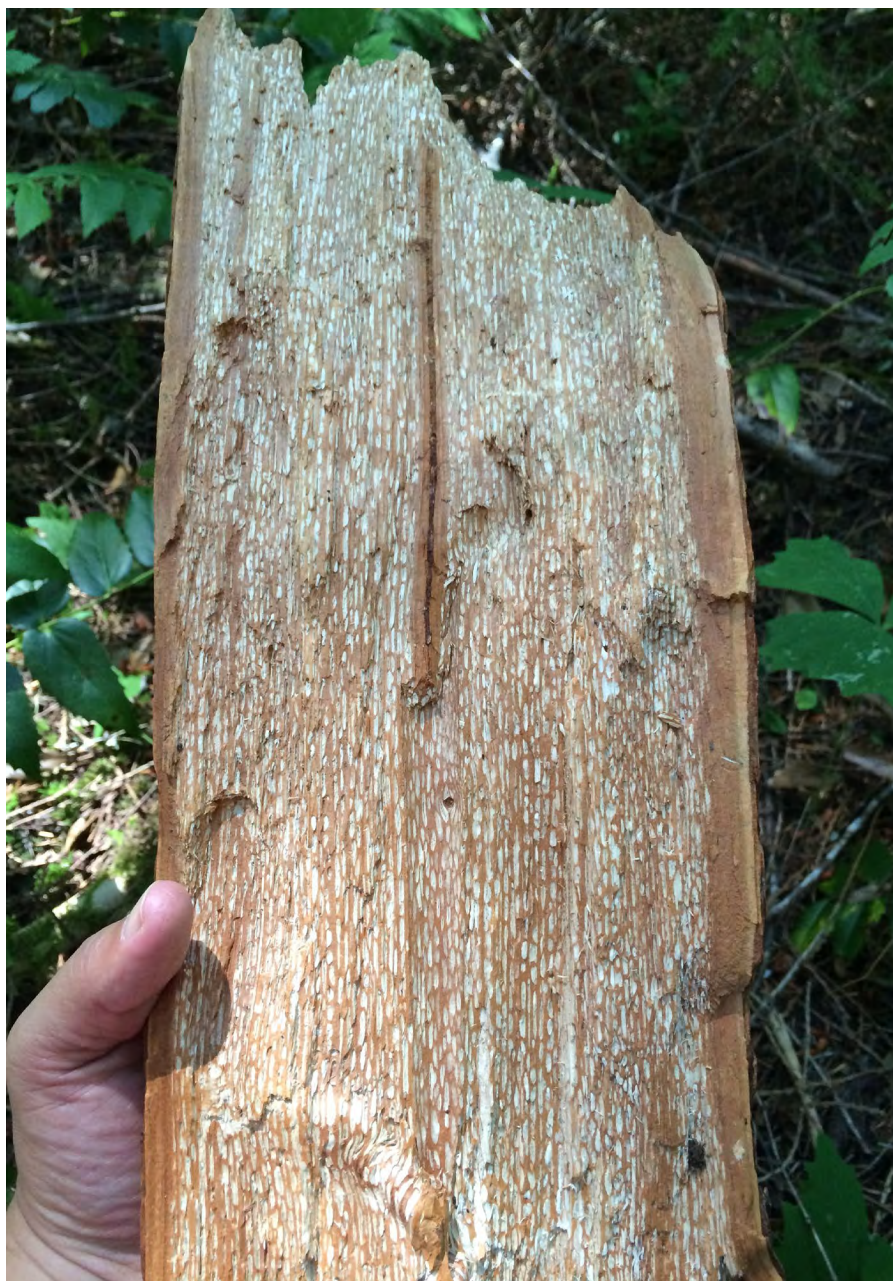
Figure A1.41—Typical Porodaedalea pini advanced decay with small white pockets surrounded by sound wood.
