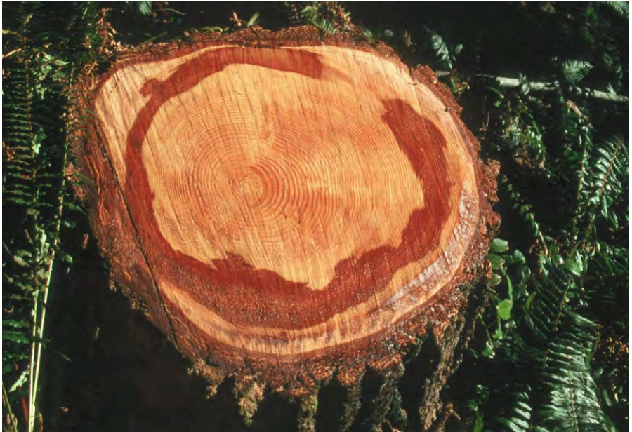
Figure A1.21—Crescent-shaped staining can be present on fresh-cut stump surfaces immediately after falling.
