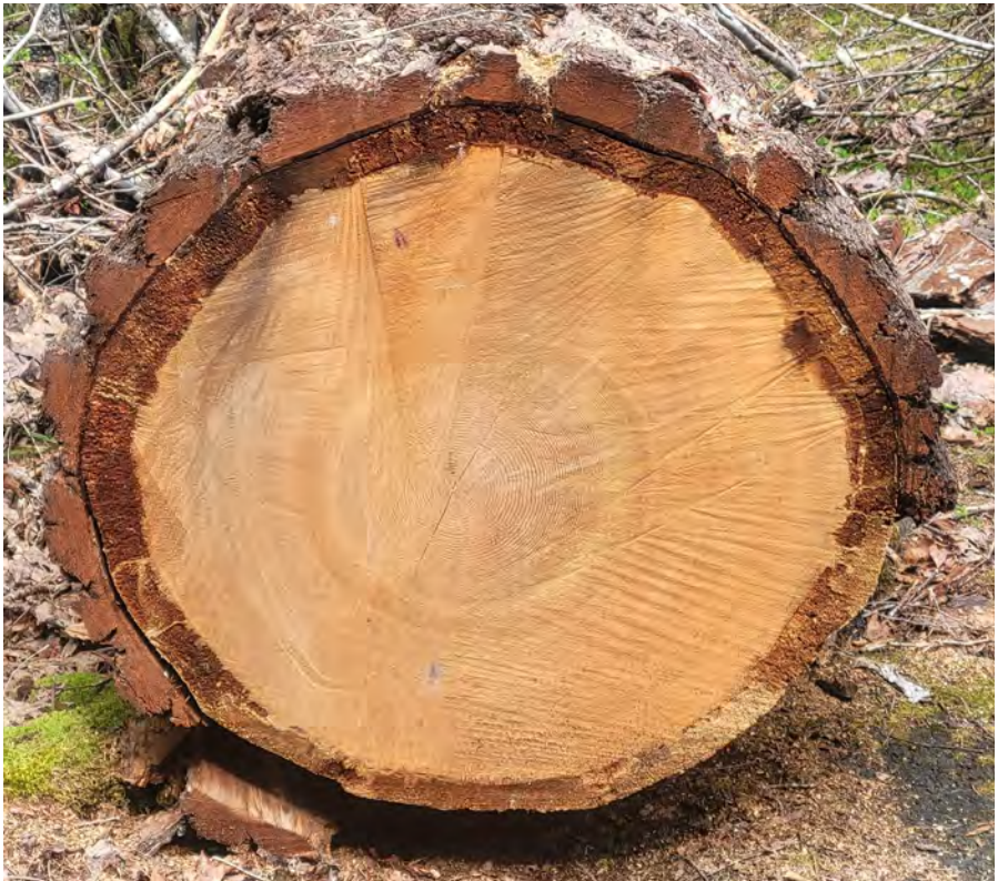
Figure 4.24—Decay in the sapwood of a tree.
