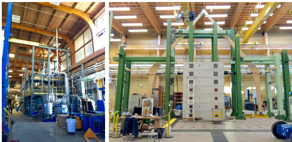
Figure 1: Active projects at the Forest Products Laboratory in Madison, Wisconsin, further our understanding of wood product applications, from manufacturing liquid nanocellulose to testing glue-laminated timber.
