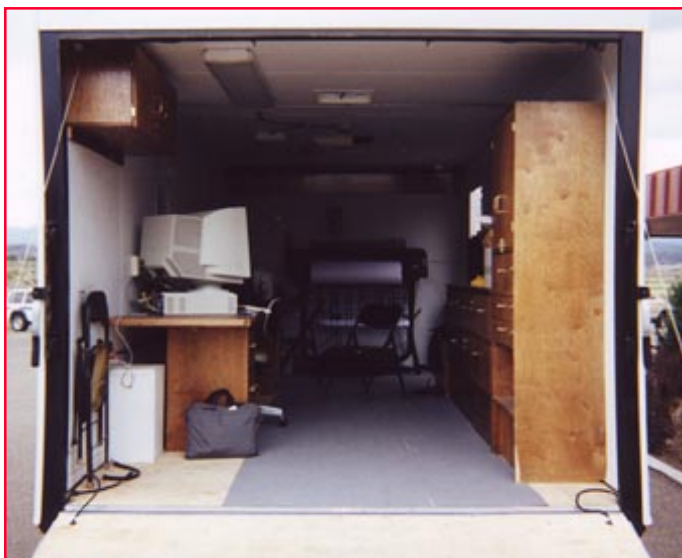
Figure 2 —Interior (above) and exterior (below) of the new mobile-mapping trailer. The large, customized trailer first saw action during the 2001 fire season. The unit can generate a fire map within 30 minutes or less from receipt of the perimeter information. Photo: Rick Connell, USDA Forest Service, Humboldt-Toiyabe National Forest, Sparks, NV, 2000.
