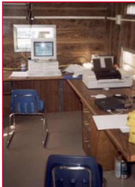
Figure 1 —Interior (above) and exterior (below) of first mobile-mapping trailer. Note computers, printer, and global positioning system inside the trailer and the generator that functioned as a supplemental power supply outside the unit. We used the converted camper trailer to develop incident action plan maps using geographical information systems and global position system applications. Photo: Rick Connell, USDA Forest Service, Humboldt–Toiyabe National Forest, Sparks, NV, 1996.
