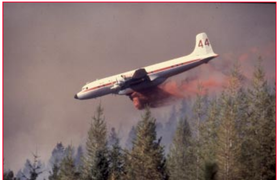
Fire retardant drop on a wildland fire. By the 2004 fire season, the Forest Service will use only gum-thickened fire retardants, less prone to evaporation and drift. Photo: USDA Forest Service.
