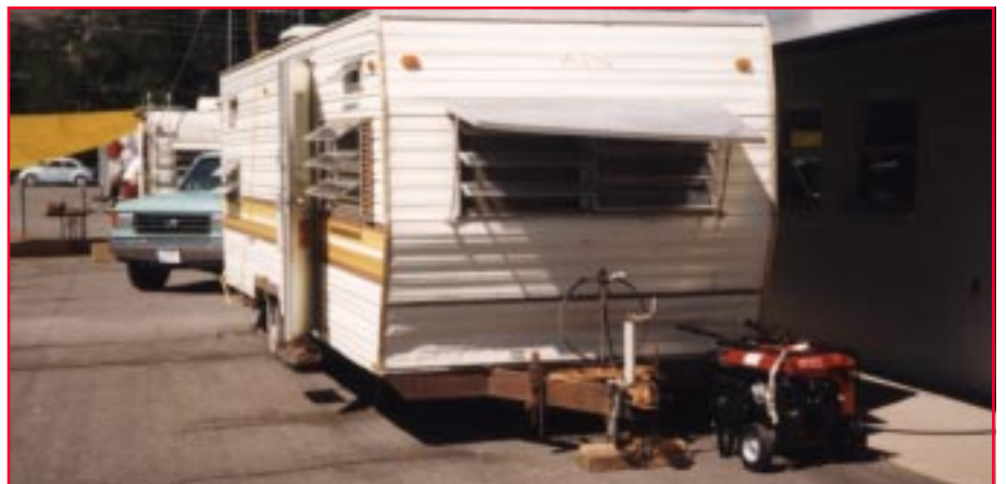
Figure 1 —Interior (above) and exterior (below) of first mobile-mapping trailer. Note computers, printer, and global positioning system inside the trailer and the generator that functioned as a supplemental power supply outside the unit. We used the converted camper trailer to develop incident action plan maps using geographical information systems and global position system applications. Photo: Rick Connell, USDA Forest Service, Humboldt–Toiyabe National Forest, Sparks, NV, 1996.
