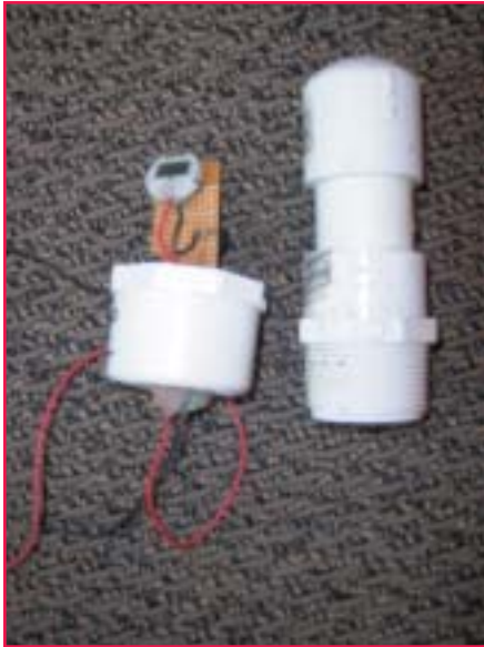
Figure 2 —The updated rate-of-spread clock is both useful and inexpensive, with parts that are easy to find. Photo: Keith Grabner, U.S. Geological Survey, Columbia, MO, 2004.
