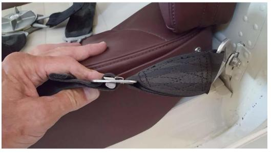
Compare the orientation of the webbing loop in the photo above...... to the PROPER WEBBING LOOP in diagram (a-1) from FAA Advisory Circular 21-34 below.
