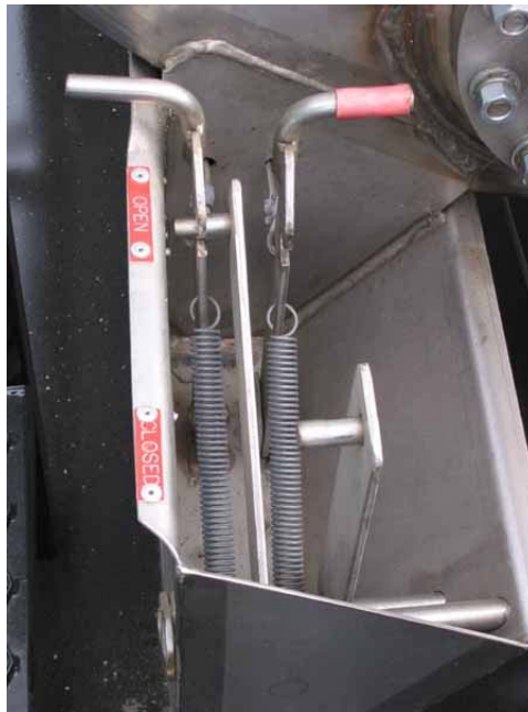
Valve Actuator Shown With Sump Valve Closed
