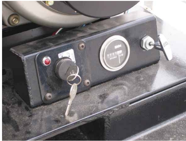
Diesel Engine Controls Throttle Shown in Idle Position
