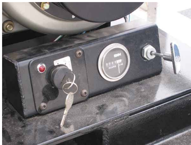
Diesel Engine Controls Shown in Start/Full Throttle Position
