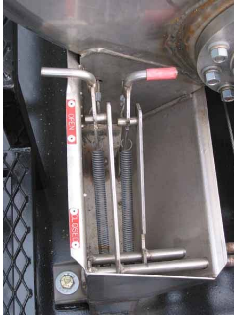
Tank Sump and Re-circulation Valve Actuators Shown With Both Valves Open
