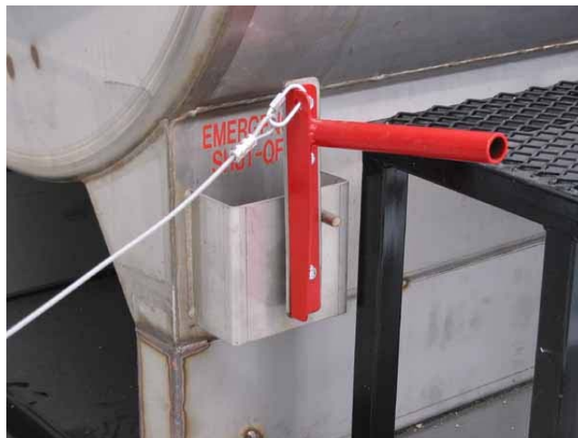
Emergency Closure Lever and Lanyard Attachment
