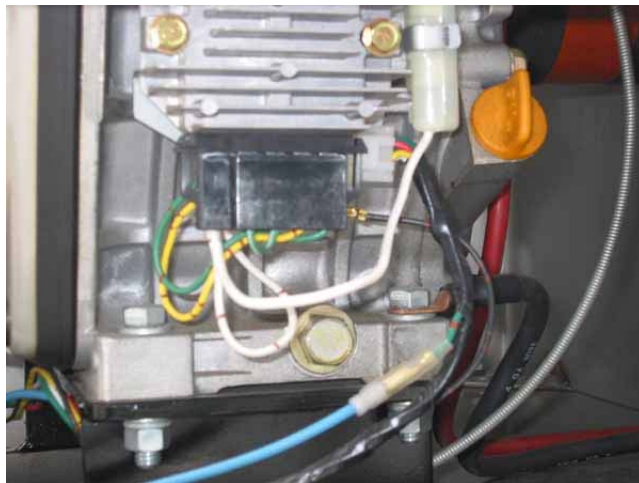
Engine Oil Drain Plug and Dip Stick
