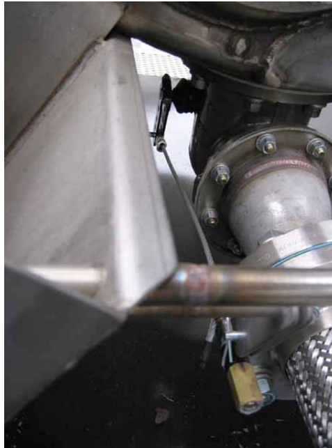
Sump Valve Fusible Link (Brass Hex Nut) and Cable
