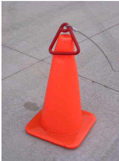
Emergency Close Lanyard Handle on Orange Cone
