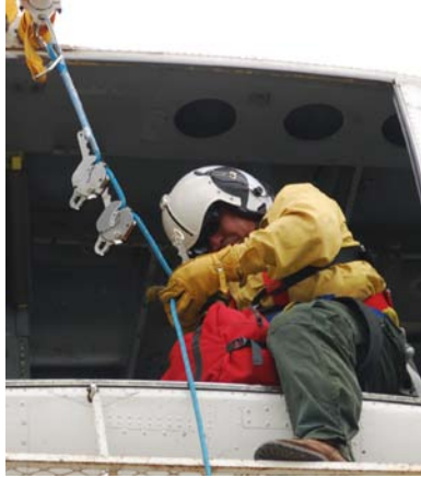
Figure 6: stacked HR-1s on rope
