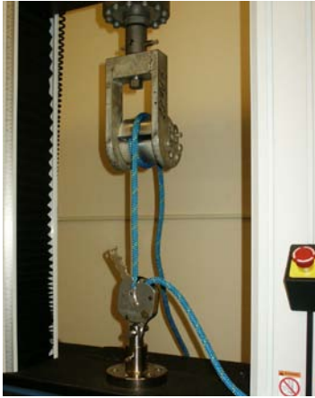
Figure 3: HR-1 static pull test
