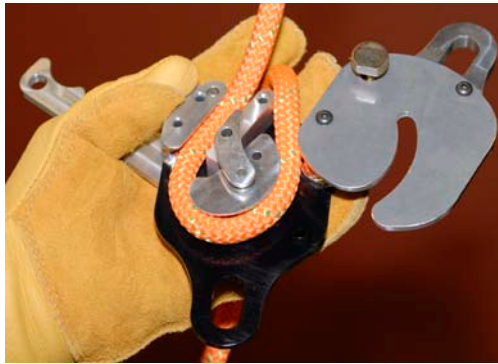
Figure 7: rigging the HR-1
