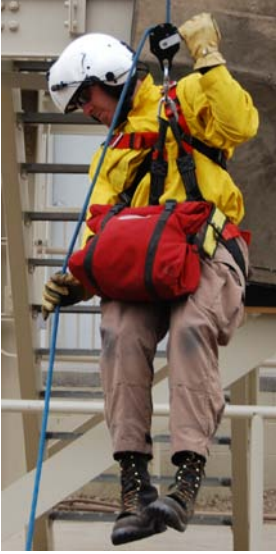
Figure 5: braking with HR-1 control lever
