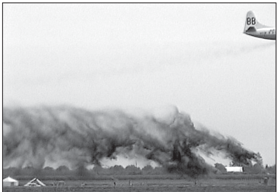
Figure 2—Retardant drop intentionally released below the safe drop height during testing.
