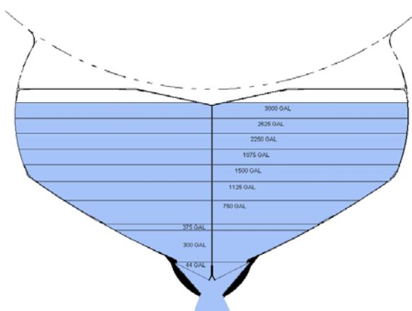
The system achieves constant flow by increasing the door opening as the liquid level falls inside the tank. For drops that require low flow rates, the doors will open a little and gradually widen as the fluid evacuates. For drops that require high flow rates, the doors open wide and have little room for adjustment. The result is the flow rate is not as constant.
