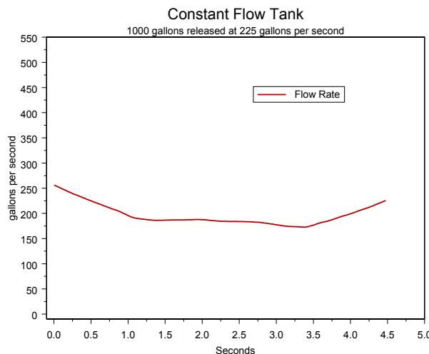
Constant flow systems have door controls that allow the delivery system to behave as a single tank. Once the drop controller establishes the flow rate, the coverage level produced remains constant over the duration of the drop. The effect of changing the volume released will only change the length of the drop, not the flow rate.
