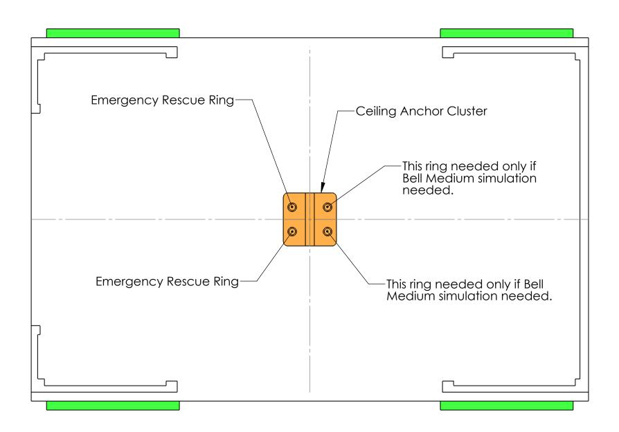
Figure 2. Ceiling and Wall Tether Anchor Installation Sites - only install the ones you need -
