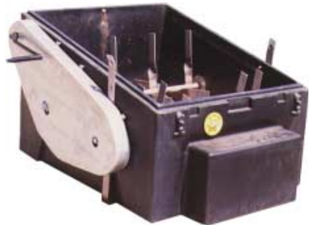
Figure 2—Modified Romtec Trailside™ Composter, top removed.
