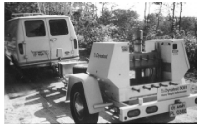
Figure 9b—FWD used at White Mountain National Forest site.
