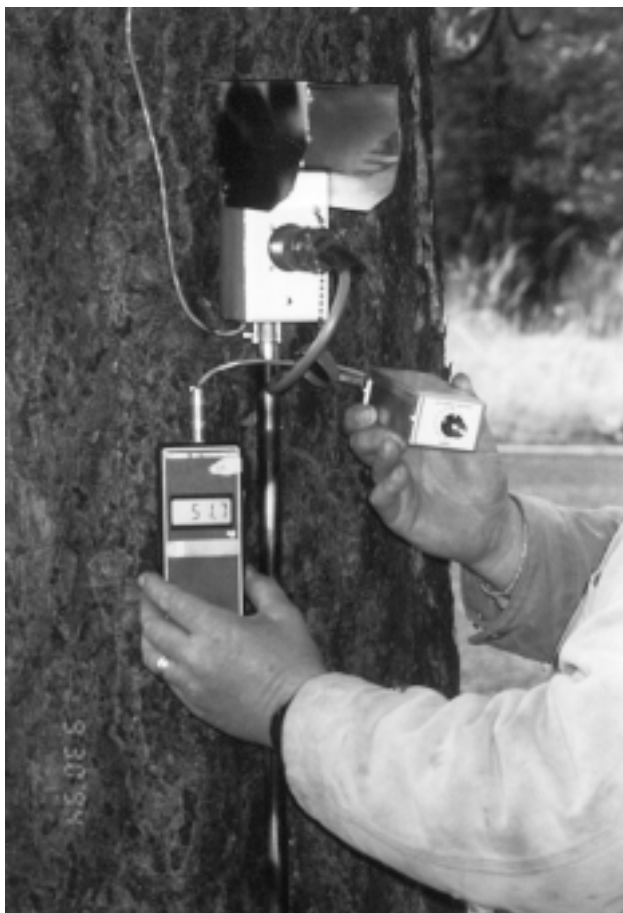
Figure 2—Taking subsurface temperatures at a typical thermistor probe installation. Sites like this exist on many national forests in the northwestern United States.
