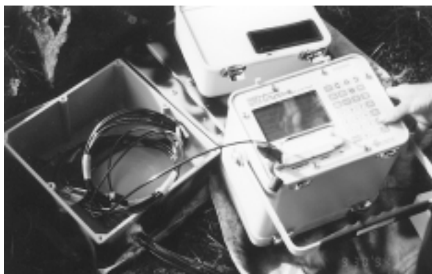
Figure 6—TRASE TDR unit taking moisture content reading from probe installed below pavement. The weather-tight utility box shown is used to protect TDR probe cable ends between readings.
