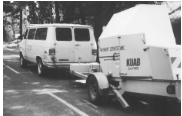
Figure 9a—FWD used at Willamette, Ochoco, and Kootenai National Forest sites.
