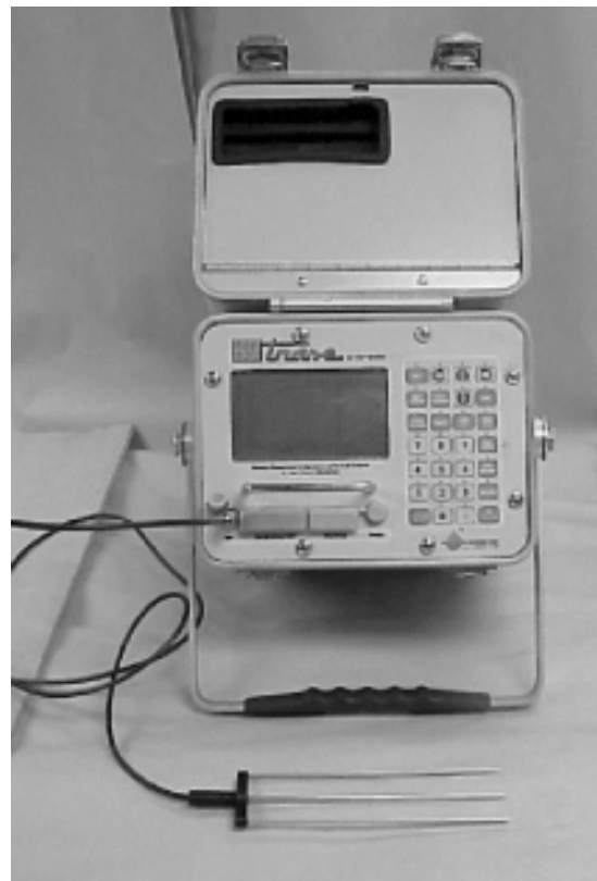
Figure 5—Soilmoisture Equipment Corp. TDR buriable probe and testing unit.
