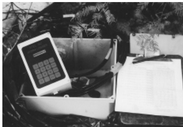
Figure 8—Vitel, Inc. RF reader is shown inside a weather-tight utility box. It is used to protect cable ends between readings.
