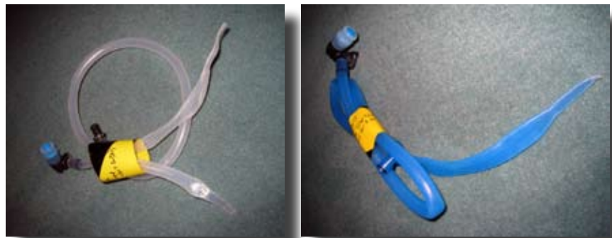
Figure 11—Structural failure of CXC and TPE bladder drinking tubes after the high temperature test.
