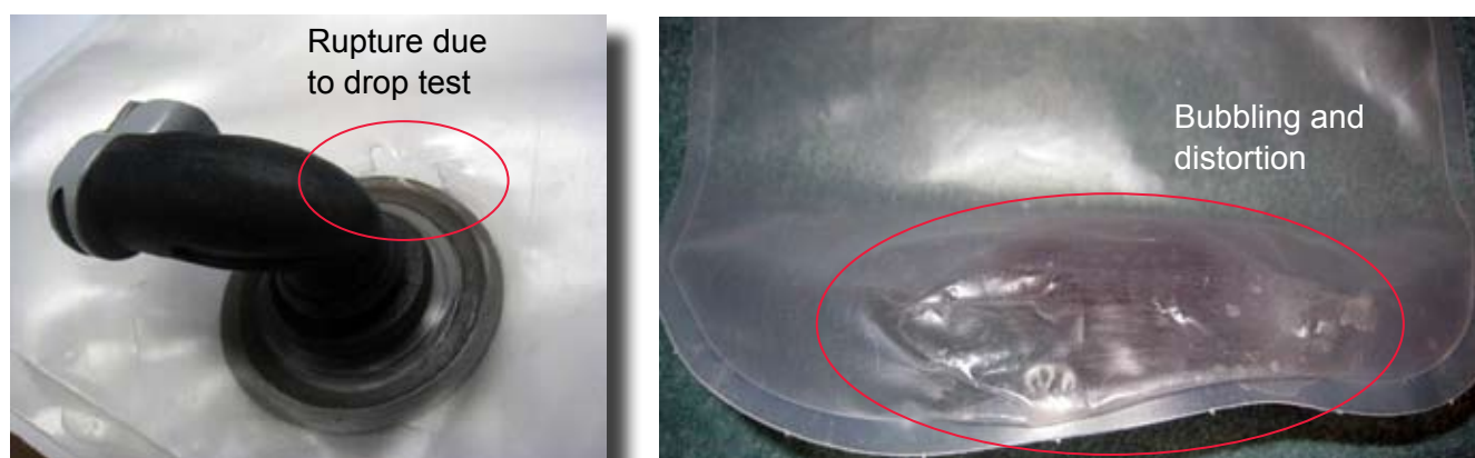
Figure 9—CXC bladder. Rupture above valve; distortion and bubbling at the bottom of the bag.
