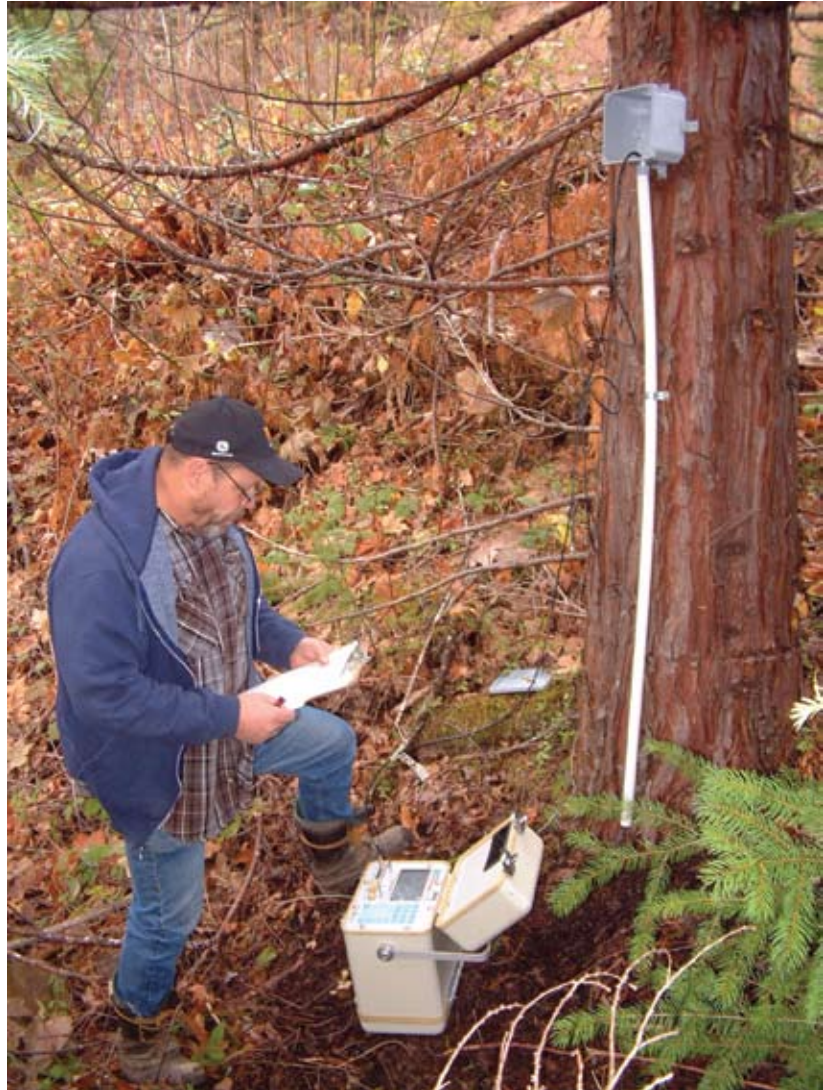
Figure 3—Reading the TDR cables.
