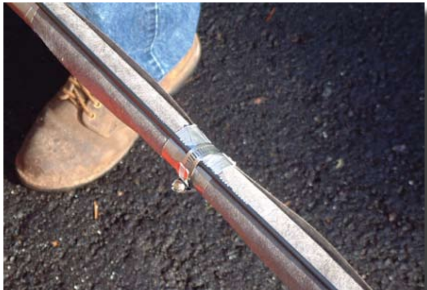
Figure 6—Hose clamp used to secure TDR cable to fabric-wrapped PVC tubing.
