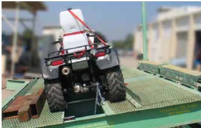
Figure A6—Some distortion in downhill tires on the Foreman ES.
