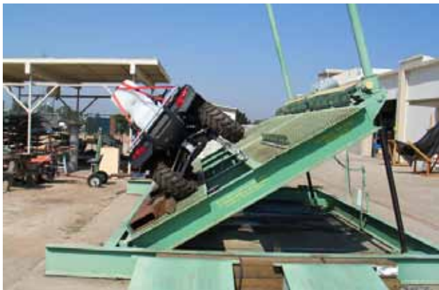
Figure A16—The Rincon rolls at 32.2 degrees.
