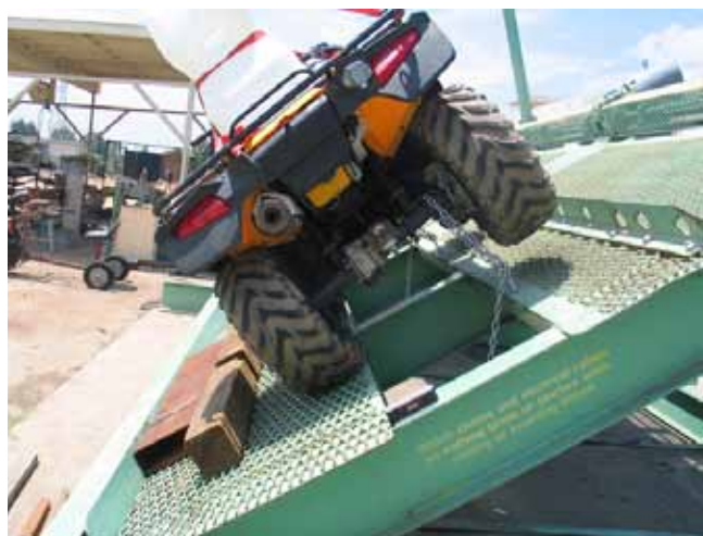
Figure A12—Rubicon ATV rolls at 34 degrees.
