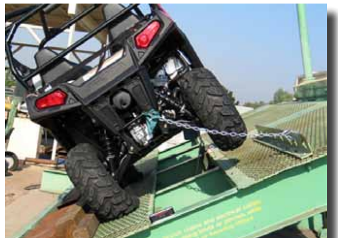
Figure A20—The RZR rolls at 32.9 degrees.
