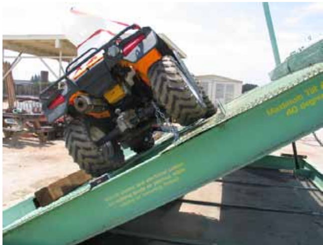
Figure A11—The Rubicon's rear wheel lifted at 27.5 degrees.
