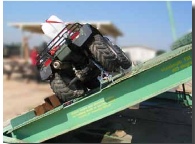
Figure A8—Foreman ES at rolling point, 30.9 degrees.
