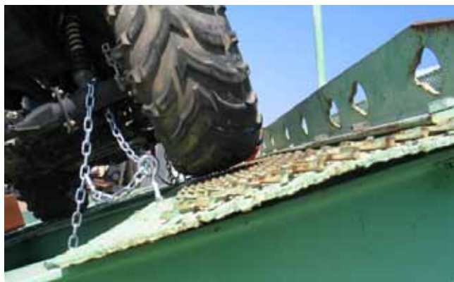
Figure A7—Foreman ES rear wheel lifted at 27.4 degrees.
