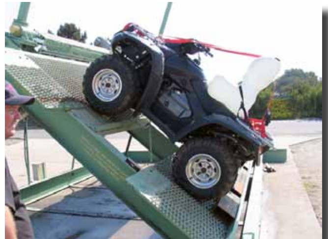
Figure A18—The Rincon tilted at 40 degrees.
