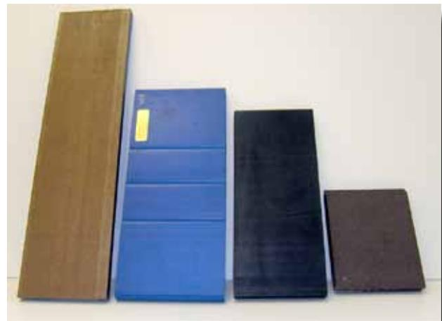
Figure 4—Fiberglass-reinforced plastic lumber example.
