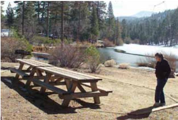
*Figure A.13—Jenks Lake picnic table made of Ipe tropical hardwood. Visitors cannot lift it and there is no carving on it; the wood is too dense and heavy.*
