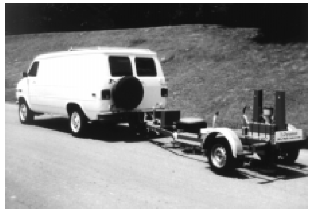
Figure 3—Falling Weight Deflectometer used to assess pavement strength recovery.
