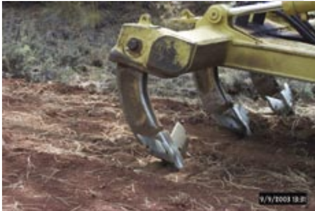
Figure 38—Larger equipment is used for deeper ripping to increase infiltration and break through water repellent soils.
