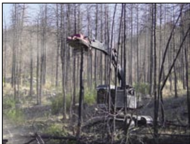
Figure 15—Mechanized equipment can quickly produce slash for effective soil cover.
