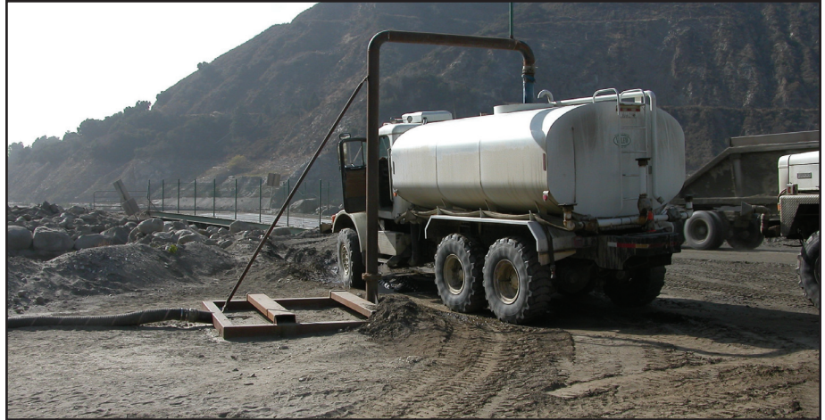
Figure 21—Standpipe used for drafting.
