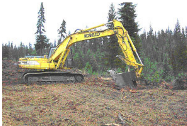
Figure 6b. Subsoiling using the SEB.
