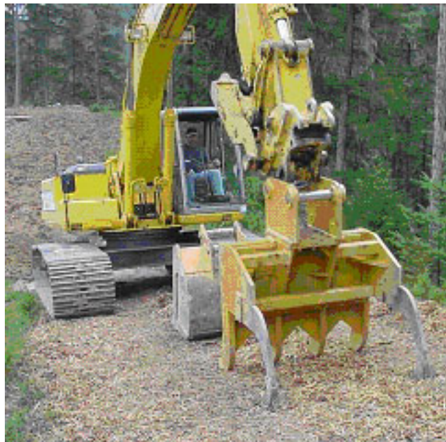
Figure 7. Close-up of coupling assembly and uncoupling from the SGR
