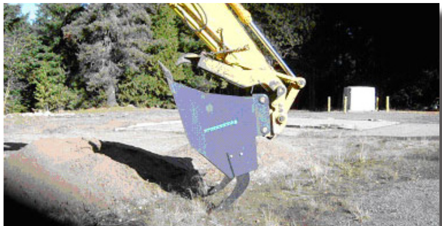
Figure 4. Side view of the prototype SEB.
