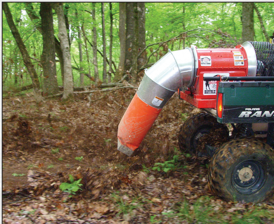
Figure 4.17—A leaf blower clears dead vegetation without disturbing the soil.
