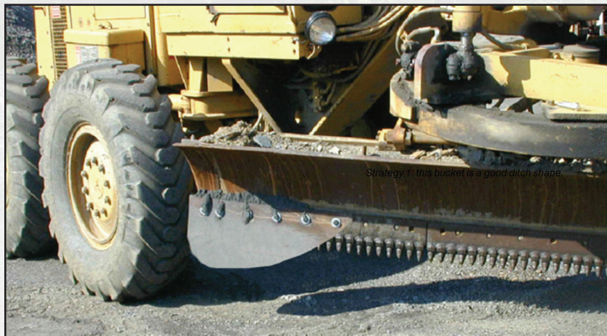
Figure 4.18—Homemade ditch cleaner for a grader.
