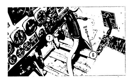
The master switch for the smoke system is located forward of the manual operation gear handle. It is a twoposition toggle switch (6) that energizes the system. The trigger switch is part of the pistol grip on the stick (7) and actuates the pump. There is no lag in the system. Smoke is immediately released whenever the trigger switch is depressed.
