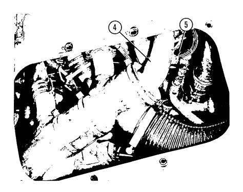
Supply lines are 3/8-inch aluminum tubing and tee into flexible steel tubing that delivers fluid to each exhaust stack (4). The exhaust stack is tapped for a fitting (5) that houses a 1/8-inch orifice fitting with a small defusing shoe. A 1/4-inch plug has been provided for cleaning the orifice with a 1/8-inch drill that is manually turned.
