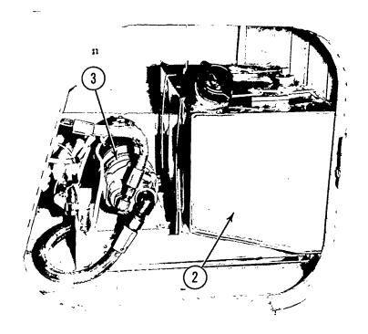
Equipment Installation. The tank (2) and pump (3) are mounted on a base that bolts down to the floor in the baggage compartment. The tank has a capacity of 9 gallons. The pump has a rating of 3-1/2 gallons of fluid at 1500 psi and is designed to handle hydraulic fluids. Each tank will run approximately 8 minutes and should produce 450 to 500 one-second bursts.
