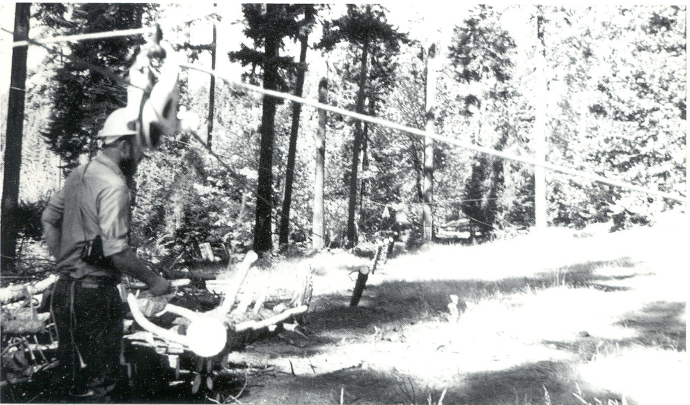
Figure 7.—Poles and chokers move toward blade mounted below the cable on a block. Note poles tied to cable, in center of photo, moving toward block and blade.
