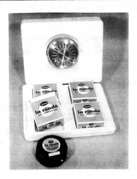
The San Dimas Equipment Development Center has field tested a new and apparently effective odor control package. It consists of a stainless steel dial control dispenser and four concentrated refill "ozitone" blocks. Twelve of these units were purchased for field testing with reported satisfactory results.
