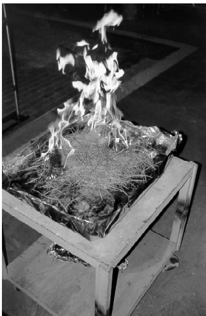
Figure 9—An example of the fire beds of pine needles used to produce smoke in the laboratory combustion chamber.
