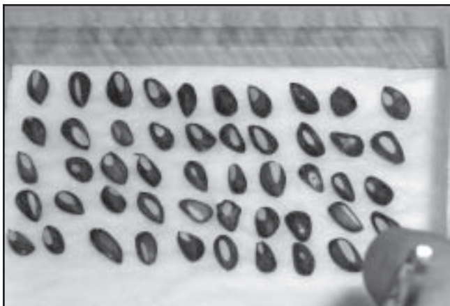
Figure 5—Closeup of seeds nicked by the prototype machine.
