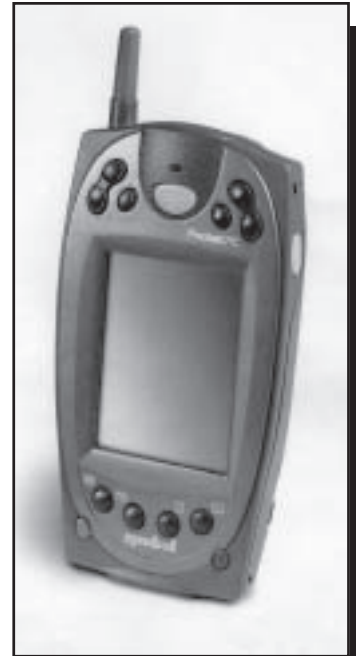
Figure 16—This wireless personal digital assistant contains an internal radio, freeing the expansion slot for a bar-code scanning card.
