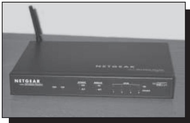
Figure 20—Access points are the preferred method of establishing radio frequency coverage.
