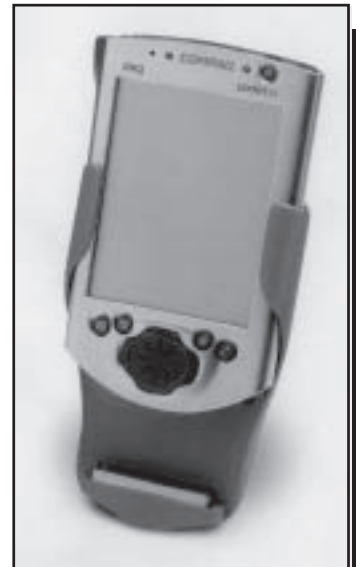
Figure 17—Most personal digital assistants have only one expansion slot. This expansion pack contains a radio, laser scanner, and separate power pack, transforming a normal PDA into a wireless bar-code scanning dynamo.
