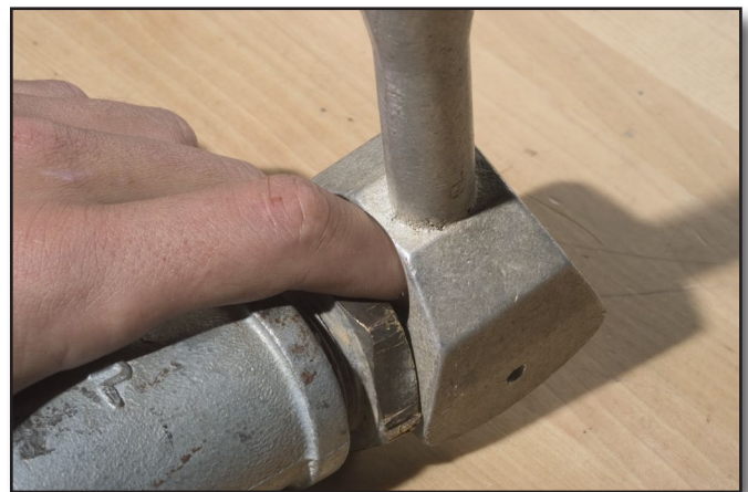
Figure 5—The handle of the modified MK-6 hydrant has room for a finger.
