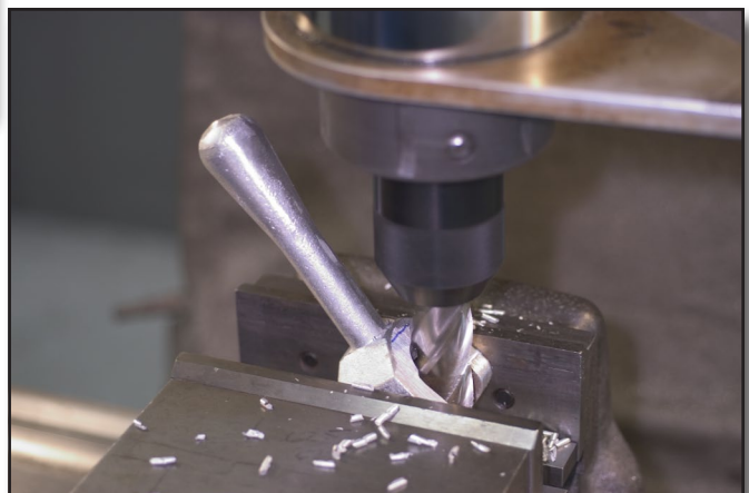
Figure 8—Mill material to the edge of the handle collar.
