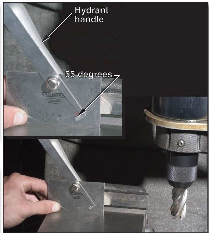
Figure 7—Use a protractor to align the centerline of the handle at a 55-degree angle.
