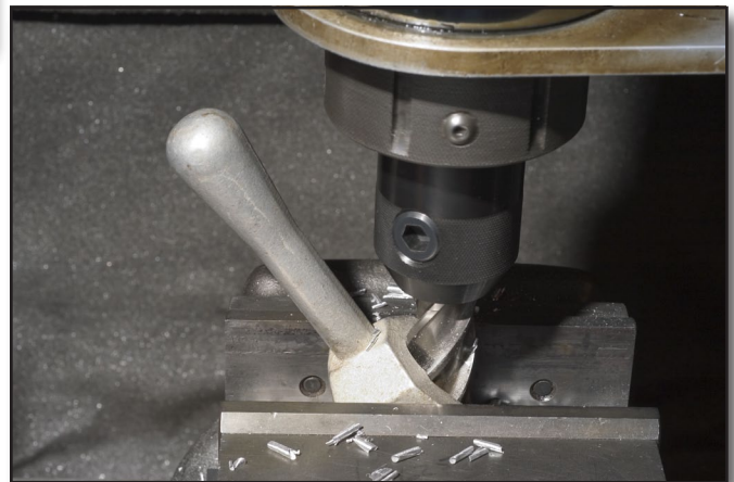
Figure 4—A milling machine was used to cut metal from the handle of the MK-6 hydrant.
