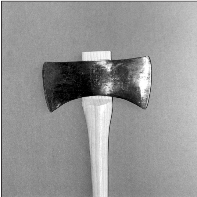
A —Size up the tool head and match it to the handle. Note that the handle protrudes excessively long through the head. Scribe it to be cut off.
