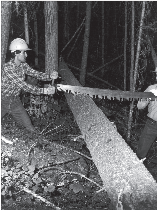
Crew members using a bucking crosscut saw.
