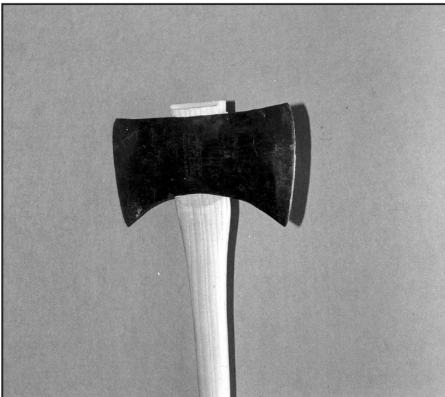
F —The wedge has been driven home with the alternate driving of the wedge and the end of the tool handle.
