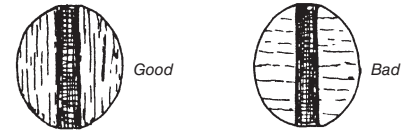
Diagram of the wedge slot and end grain of ax handles.
