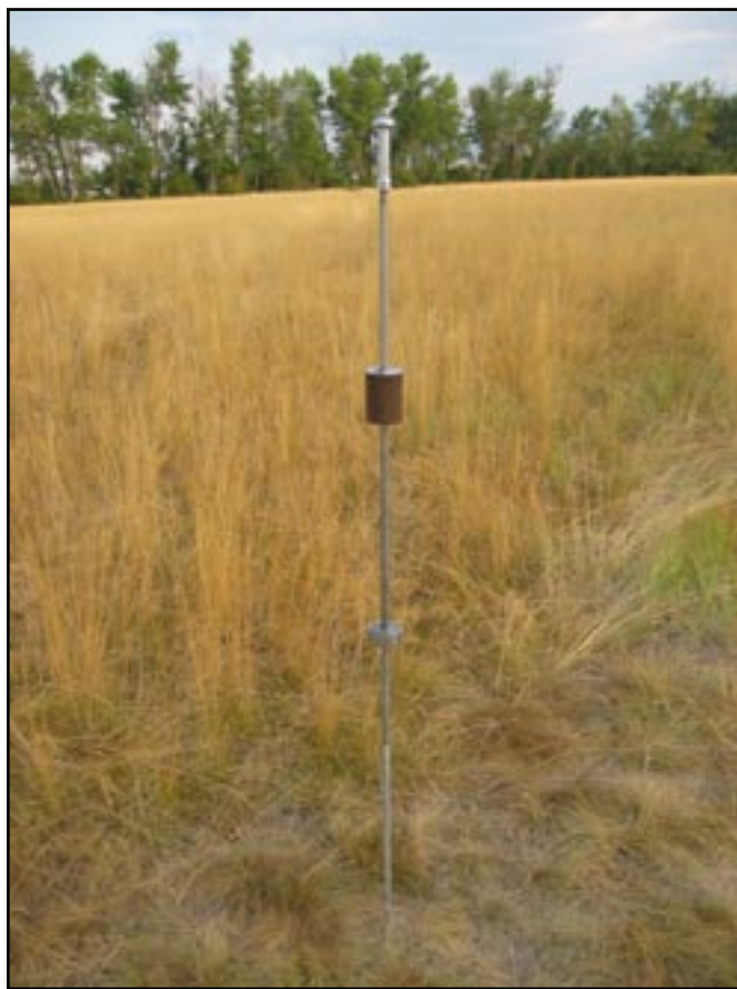
Figure 12—The slide hammer on a dynamic cone penetrometer is dropped from a given height for a given number of times and the probe's depth is recorded. This device is less expensive ($1,200 to $2,500) than the hand-held electronic cone penetrometers, but it takes much longer to use in the field and the cone index must be calculated after use.
