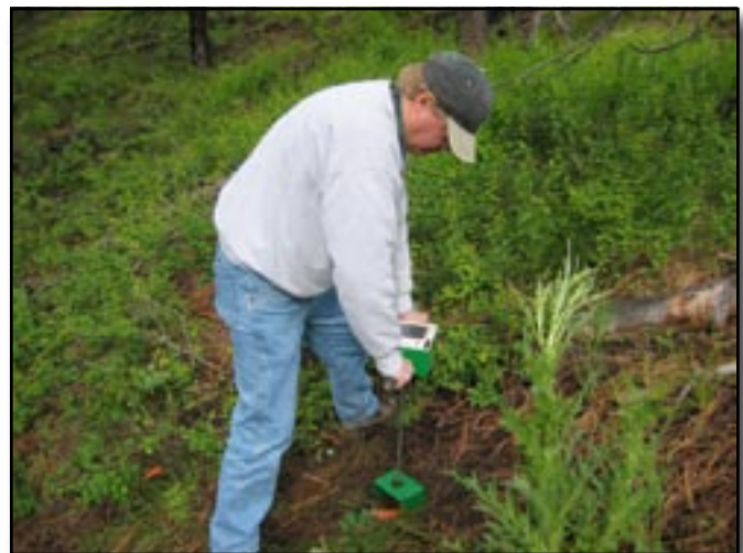
Figure 5—Penetrometer testing in the Boise National Forest near Idaho City, ID.
