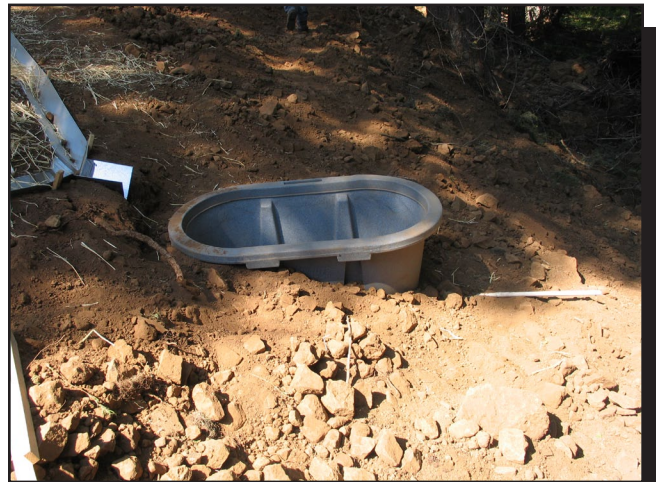
Figure 9—These tanks collect sediment and water from the test plots.
