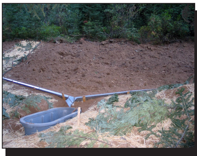
Figure 3—A plot with the bare ground exposed. Erosion on plots with bare ground will be compared to that on plots with erosion control treatments.
