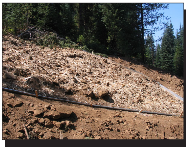
Figure 2—A test plot covered with wood shreddings to reduce erosion.
