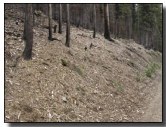
problems caused by erosion. Meanwhile, trees cleared from road rights-of-way need to be burned or chipped to reduce fire hazard. Could small-diameter trees cleared from road rights-of-way be shredded and used as mulch for erosion control? Engineers at MTDC were asked to evaluate this possibility.
