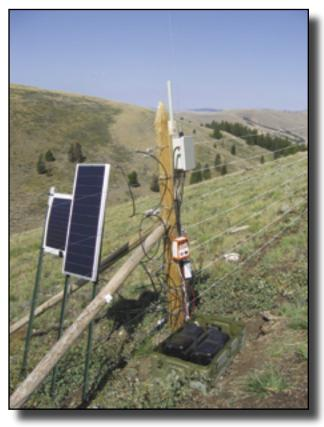
snow and high winds make it a worst-case testing ground for weather conditions. The fences installed consisted of two battery-powered electric fences with solar charging systems, and one plastic mesh fence.
