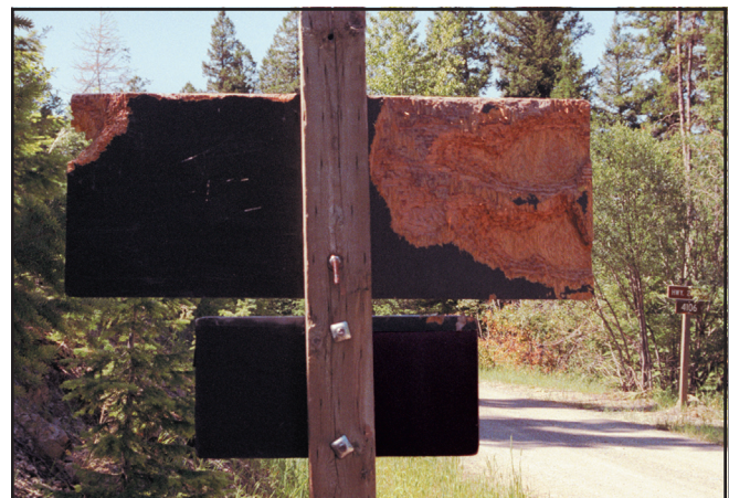
Figure 3—The back of the Dry Creek road sign in July 2004. The treated (left) half of the sign shows no further damage, while the untreated (right) half has been chewed severely.
