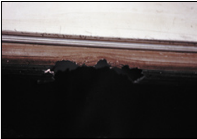
Figure 7—This hole was the only damage to the door seal 8 months after the habanero coating was applied.
