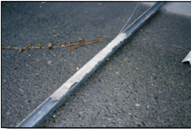
Figure 6—Chipmunks severely damaged overhead door seals, which were replaced every year or two at the maintenance shop in the Mount St. Helens National Volcanic Monument.
