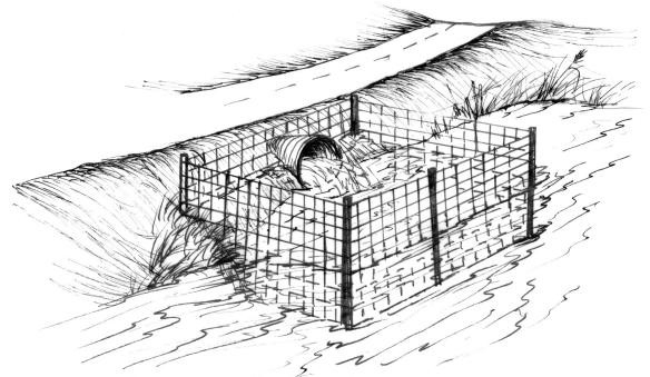
Figure 7-A fence built from panels of metal mesh can keep beavers from reaching a culvert.-Drawing by Dr. Jeanne Jones
