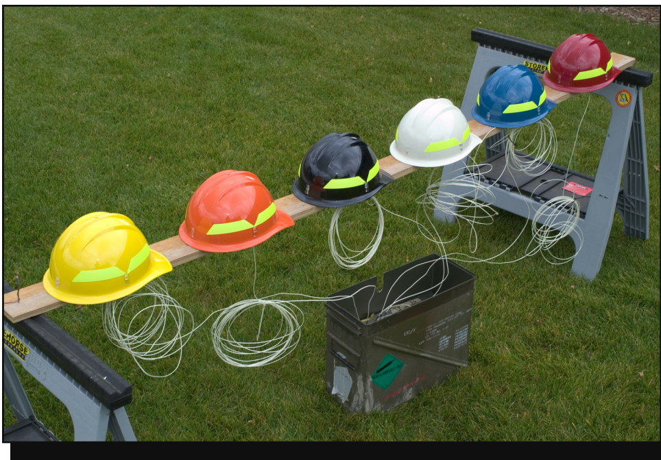
Figure 1—The six hardhats on the test rack were wired to a datalogger that recorded the temperature inside the hardhat every 5 minutes.
