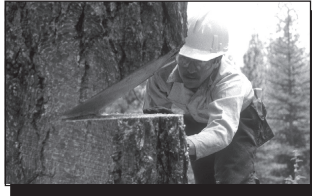
Figure 4-23—The sloping cut is a 45-degree angle.
