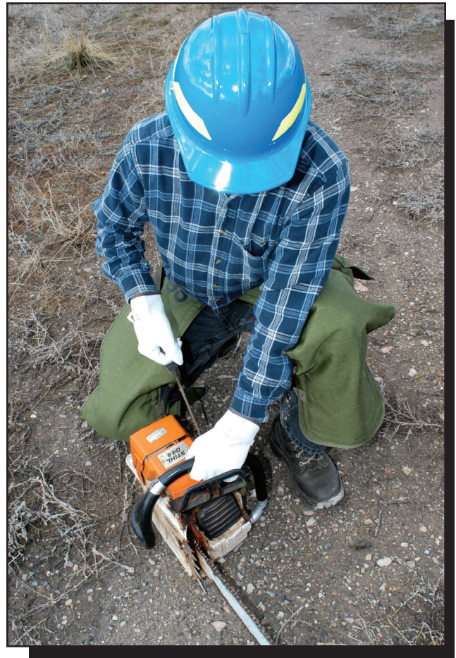
Figure 3-17—Start the saw on firm ground.
