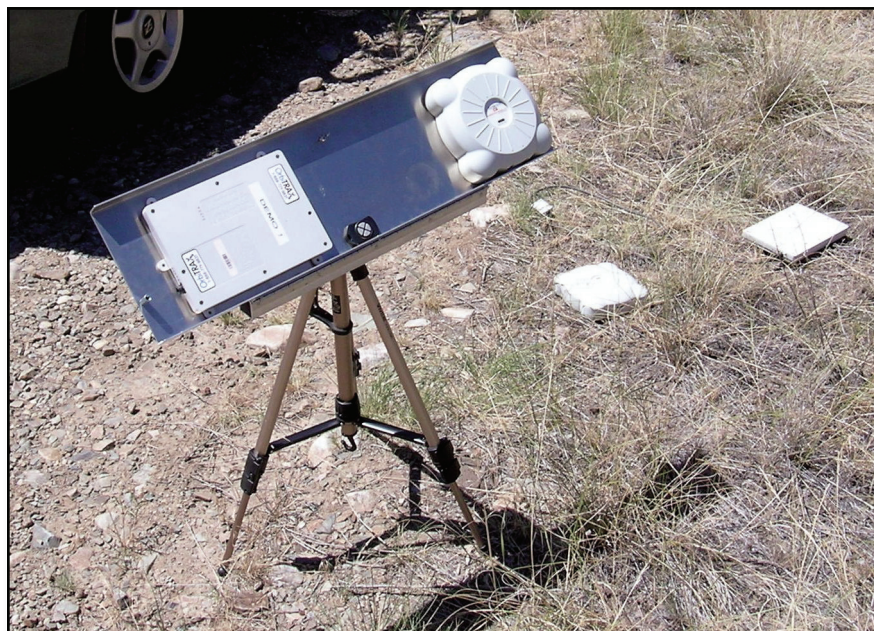
Figure 4—Axonn AXTracker (left) and Guardian Mobility Tracer (right) transmitters were mounted on a stand that was tilted 45 degrees north during some of the tests. In northern regions, transmitters tilted to the north would be more likely to have difficulty making satellite transmissions.
