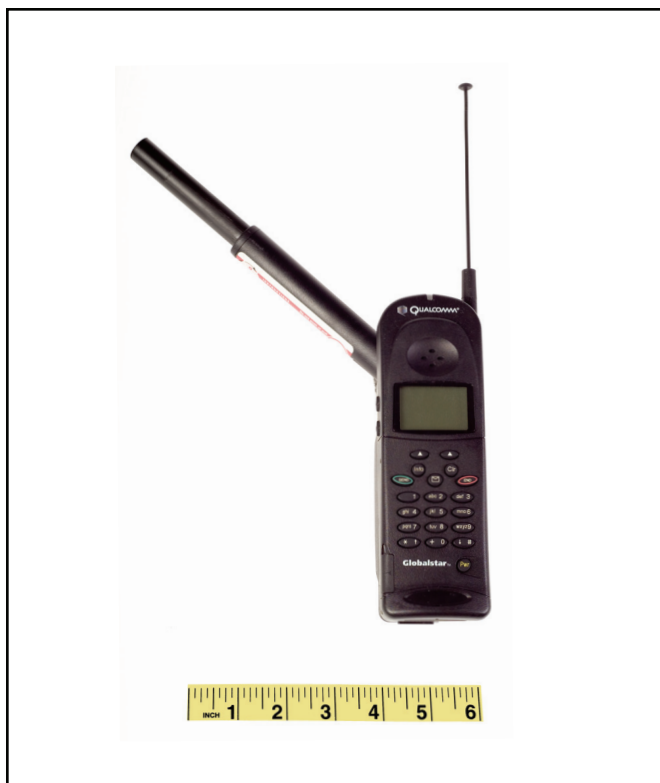
Figure 2—A satellite phone provides duplex (two-way) communication.
