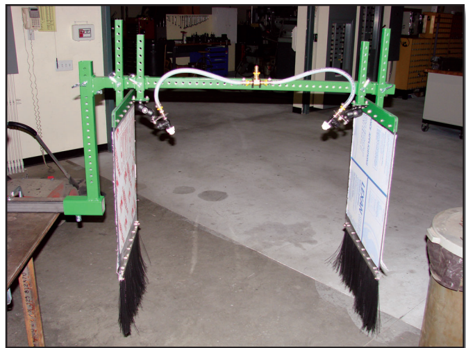
Figure 3—The new design allows both the nozzles and the shield to be adjusted, providing good spray coverage on weeds and grass while keeping overspray off desired crops.
