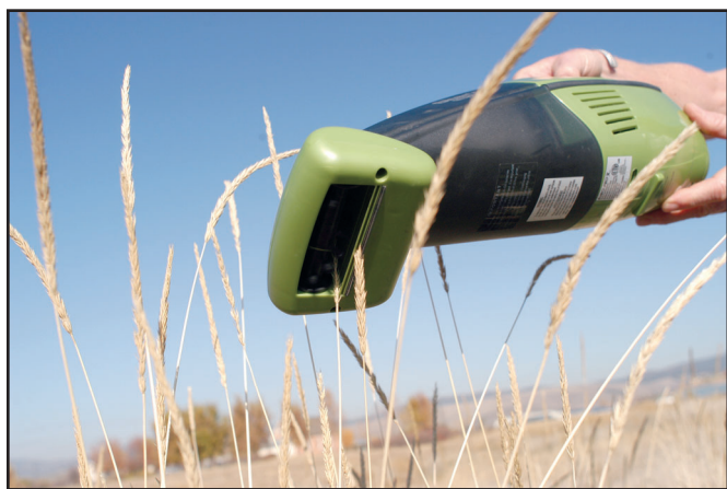
Figure 6—Attempting to collect seed with the Euro-Pro Shark hand-held vacuum.
