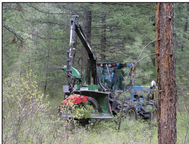
Figure 5—A self-feeding wood chipper attached to a tractor.
