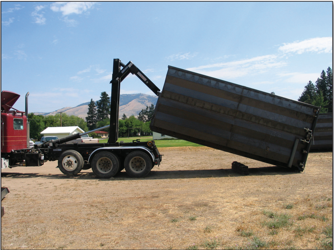
Figure 6. A slash container roll-on/roll-off bin for collecting shredded wood.
