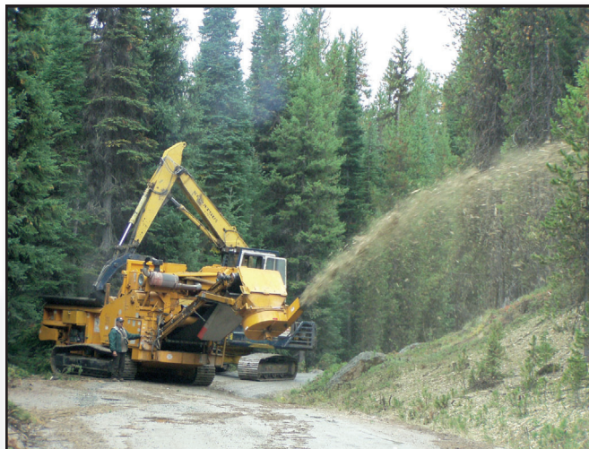
Figure 4—A horizontal shredder fed by a trackhoe can shoot shredded material into the woods for erosion control.
