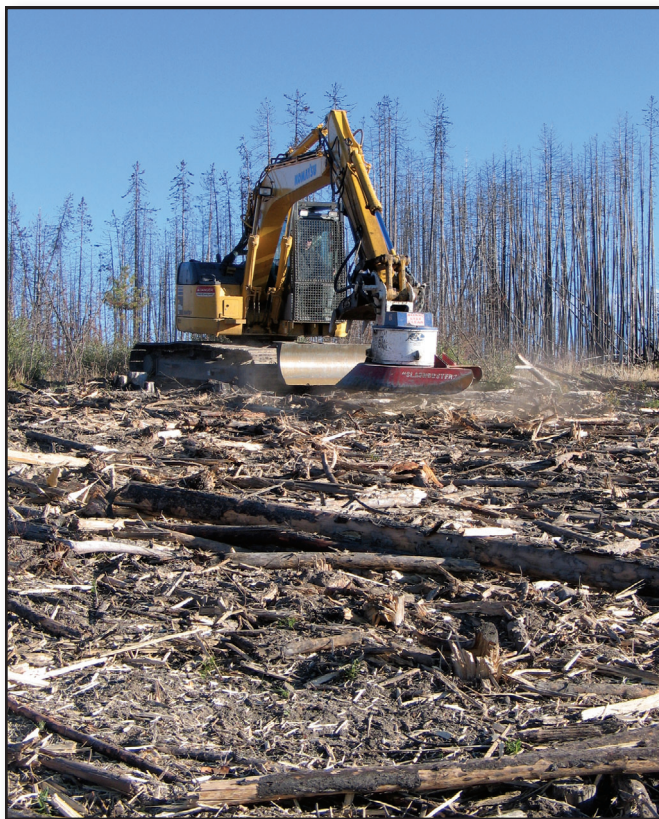
Figure 3—A trackhoe with a mastication attachment used to shred material in place.
