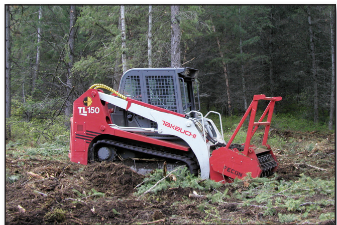
Figure 2—A mastication attachment on a small skidsteer.
