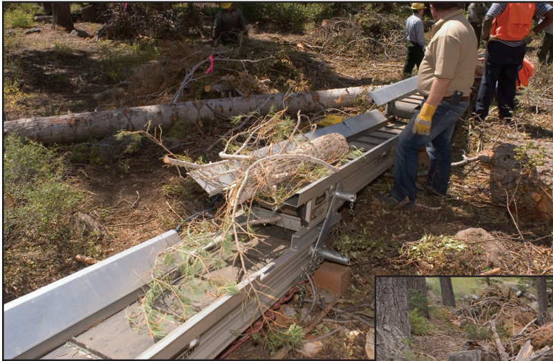
Figure 4—Even though the conveyor sections were overlapped and side extensions were installed, slash was difficult to keep on the conveyor.
