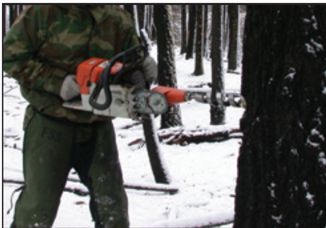
Figure 4a—Auger bits can be attached to chain saw motors and used to bore holes in trees, allowing explosives to be loaded internally.
